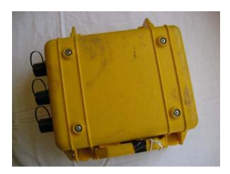
Remove 4 screws from base of unit (ensure that the metal and rubber washers are stored in a safe place)
