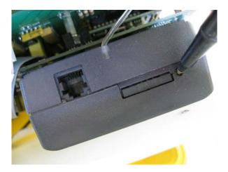
Use a pointed object (eg ballpoint pen) to press the yellow button on the GSM module to release the SIM card holder
