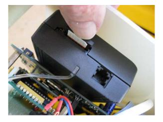
Reinstall the SIM card holder (ensure the SIM card is seated fully into the holder and that the holder is fully inserted)
