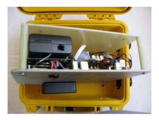
Carefully ease inner assembly out of the outer case and position as shown (avoid any tension to the wiring between the outer case and the inner assembly)
